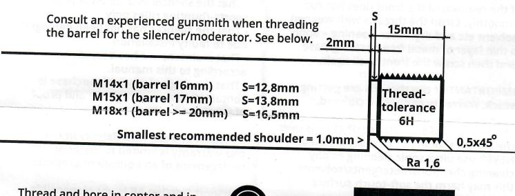
Thread and bore in center and in line with the silencer.
